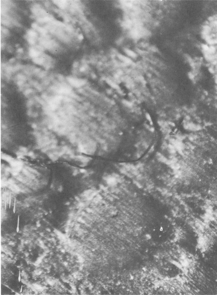
FIG. 8—Red acrylic fiber in situ in fiber-plastic fusion shown in Fig. 6.
